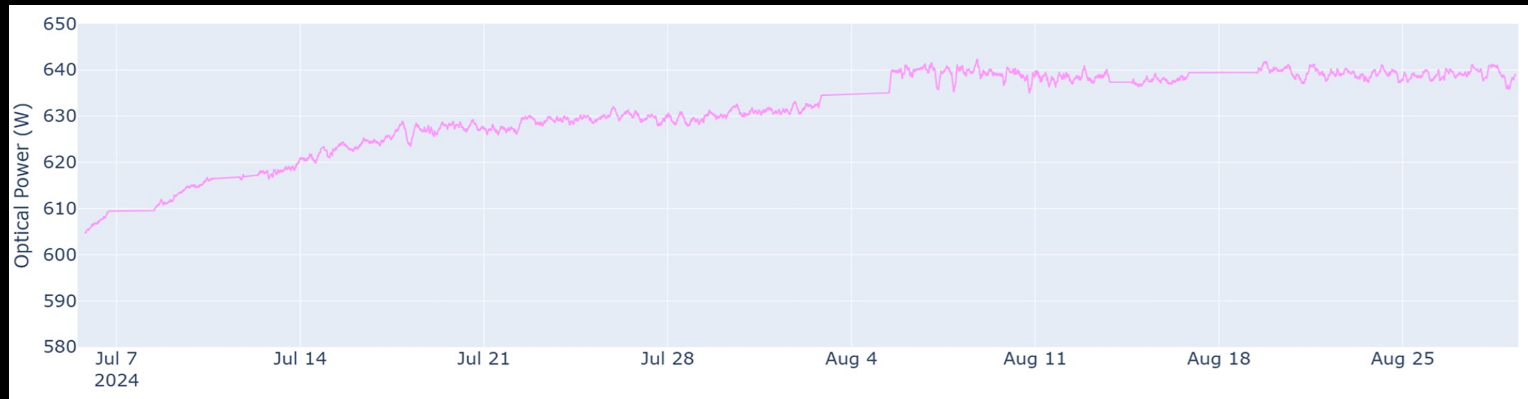
Optical power over the course of 1,095 hours of lifetesting at 25°C
